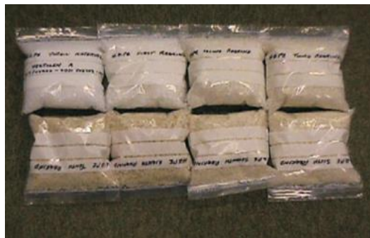
Figure 2: Quality Degradation From Recycling HDPE: Colour change of HDPE after ten processes of recycling. Quality of material decreases from upper left corner preceding clockwise. Source:(Goodship, 2007)
