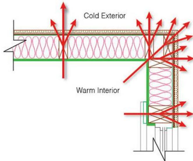
Figure 12. Corners provide a larger surface area through which heat can be transferred. Image: AIA/Architectural Record Continuing Education Program<sup>12</sup>
