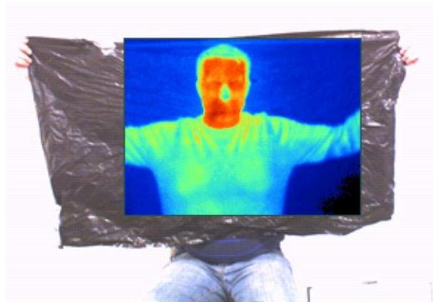
Figure 3. Infrared radiation transmitted through an opaque sheet of plastic. Image: MoistureView<sup>3</sup>.
