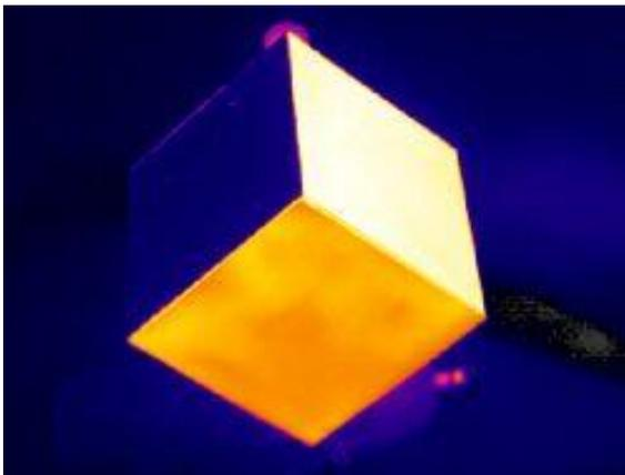
Figure 4. A Leslie cube. To demonstrate the effects of surface emissivity, each side of this cube was coated with a different material. Although each side appears different when viewed through a thermal camera, the internal temperature is the same.
