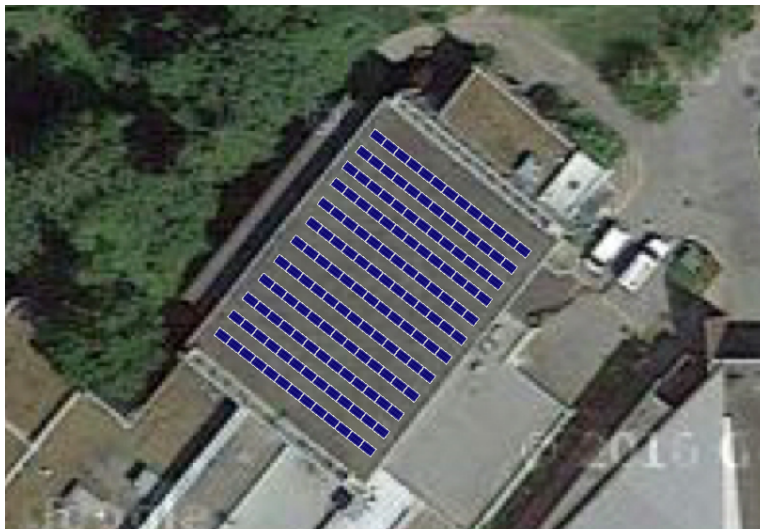
Figure 5 – Solar Thermal System Layout at Renfrew Park CC
