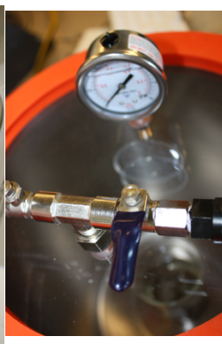
Using a vacuum chamber to penetrate roots with glomalin-dissolving solution
