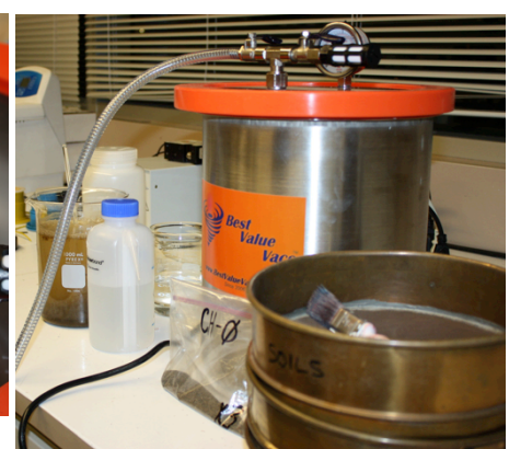
Using a vacuum chamber to penetrate roots with glomalin-dissolving solution
