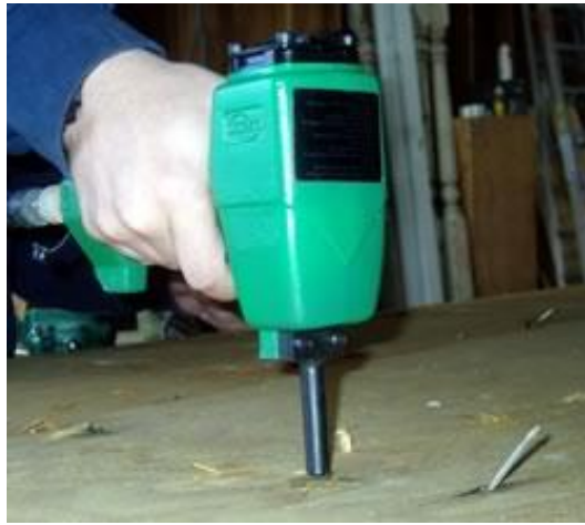
Figure 9 A pneumatically-powered de-nailer tool
