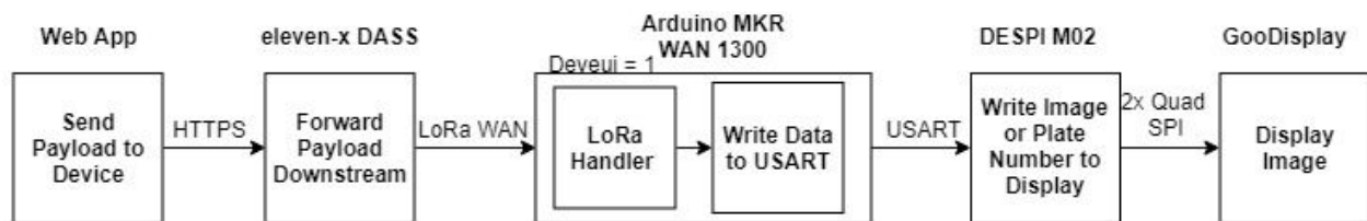
Figure 6.1: Downstream Payload Flow
