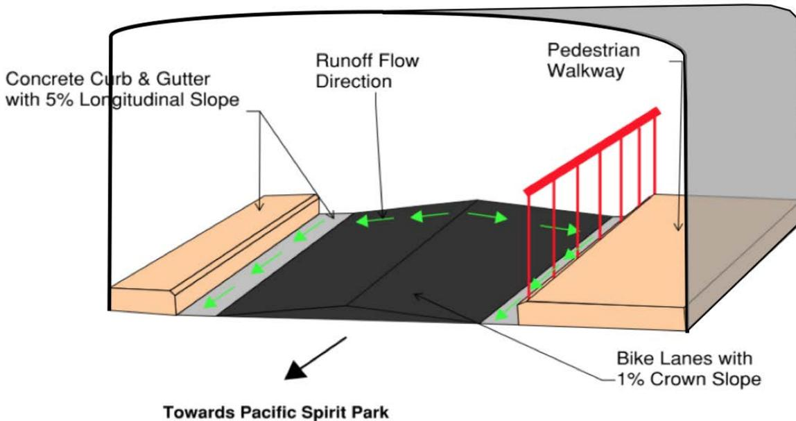
*Figure 13 - Overland Flow Within Tunnel Drainage System*
