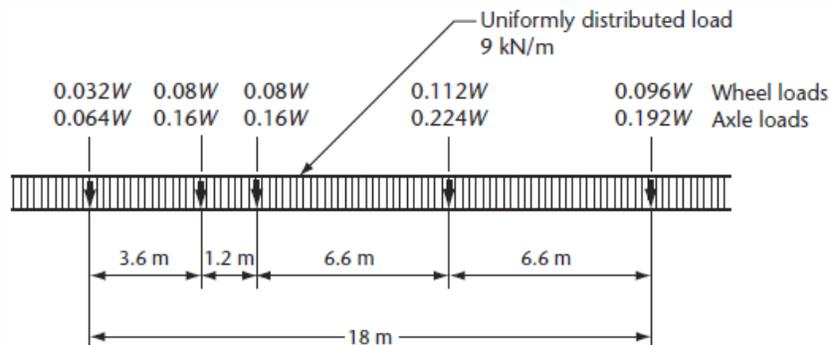
Figure 5 - Factored Truck Load with Distributed Loading
