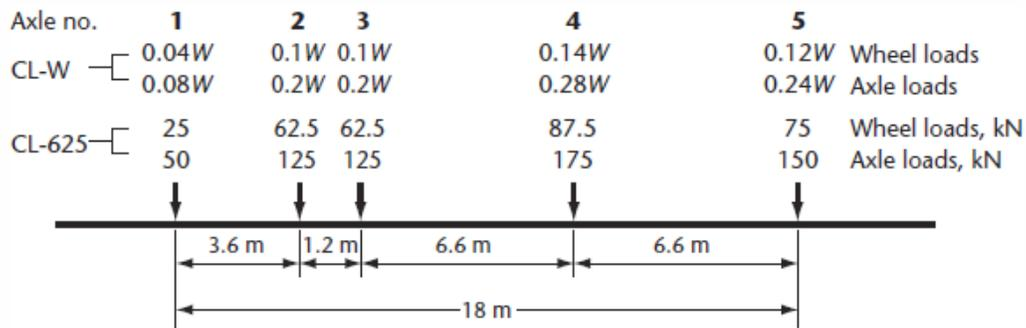
Figure 4 - CL-625 kN Truck Loading Case
