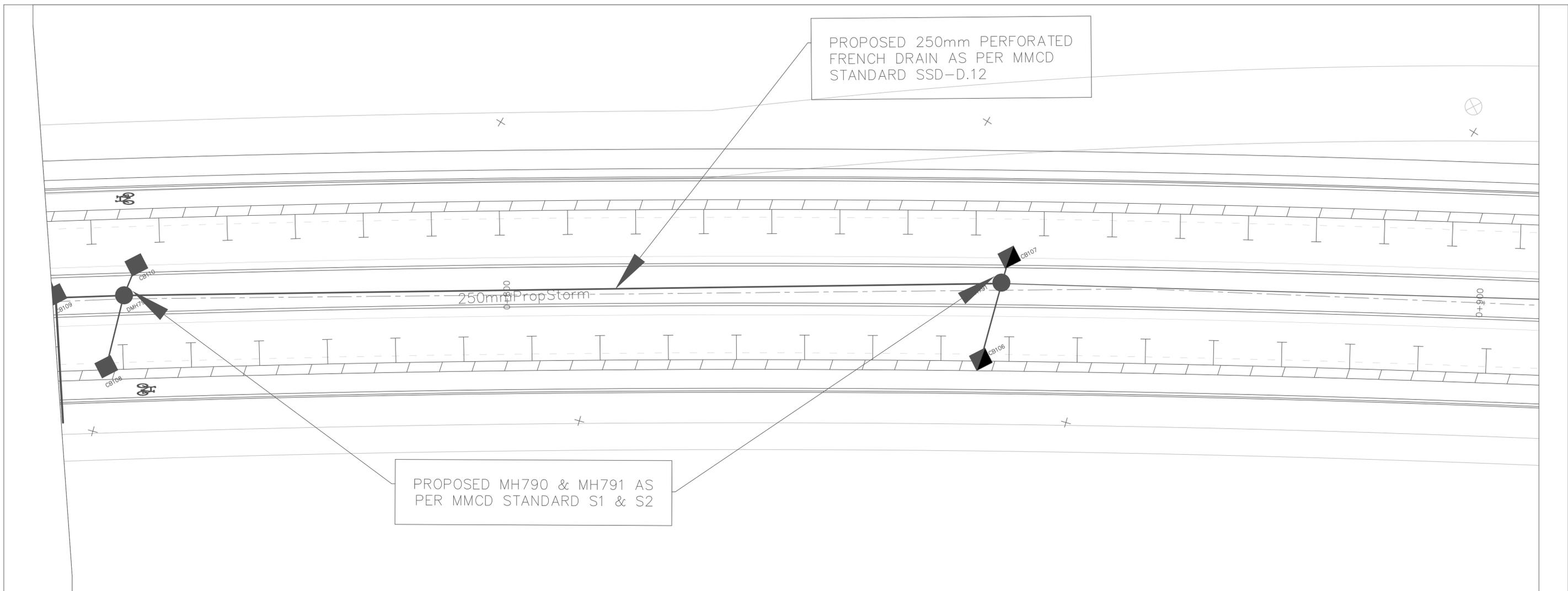
PROPOSED 250mm PERFORATED FRENCH DRAIN AS PER MMCD STANDARD SSD-D.12
