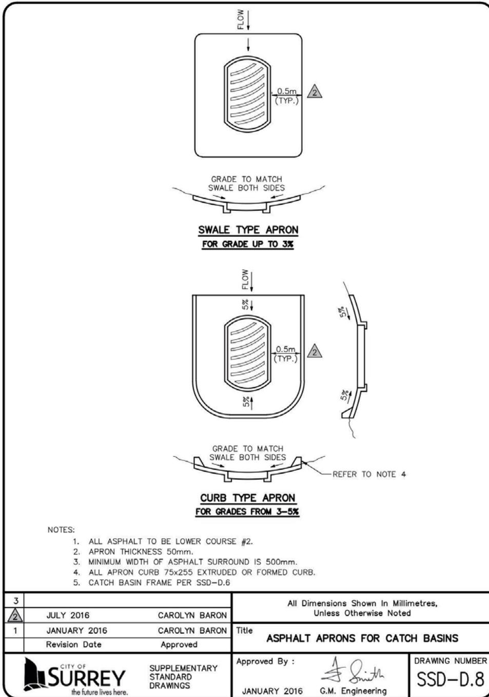
Figure E - 2 - Asphalt Aprons For Catch Basins (Supplementary Standard Drawings, 2016)
