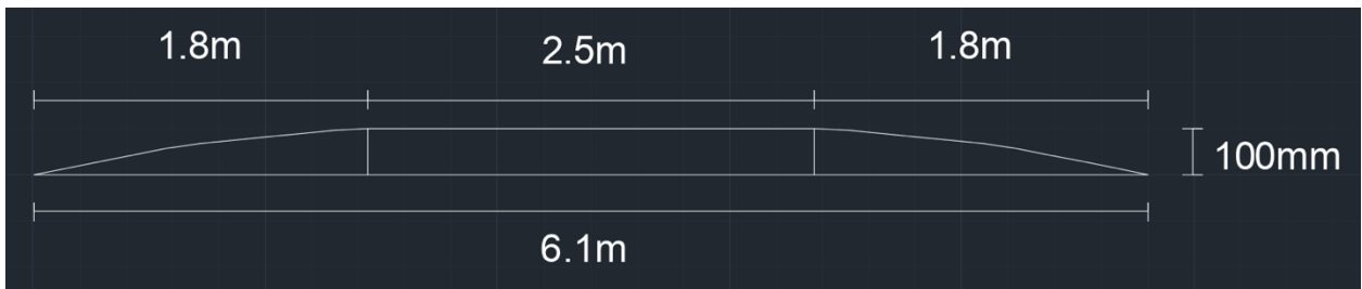
Figure 11: Raised Crosswalk Cross-Section
