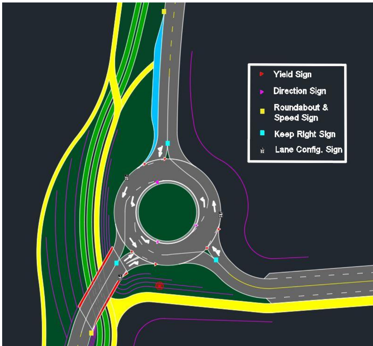
Figure 19: Roundabout Design with Signage & Pavement Markings
