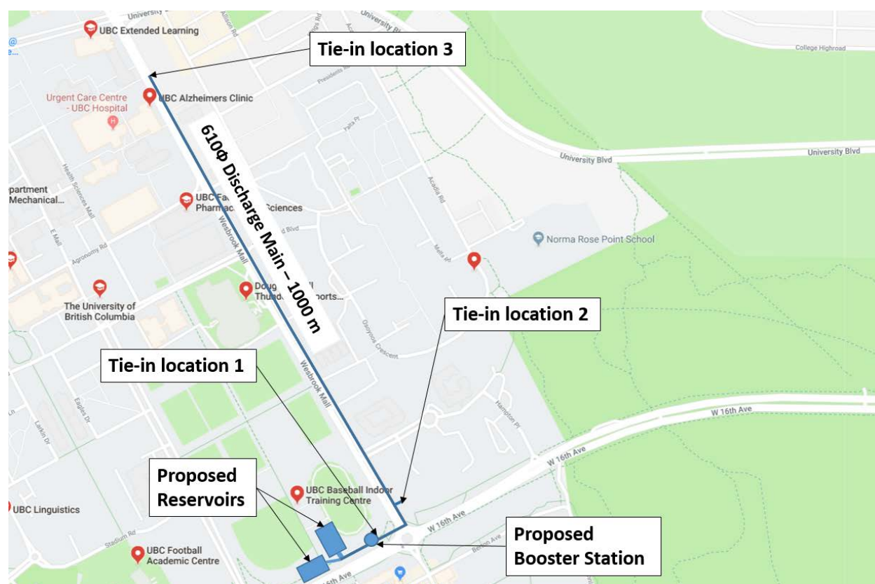
Figure 8: Discharge main alignment and proposed tie-in locations
